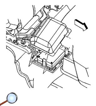
2. Remove the protective cover from the vehicle communication interface module (VCIM).
